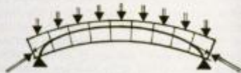
Compression structure alone: a masonry arch wedged into position along line of compression in a reversed catenary curve
